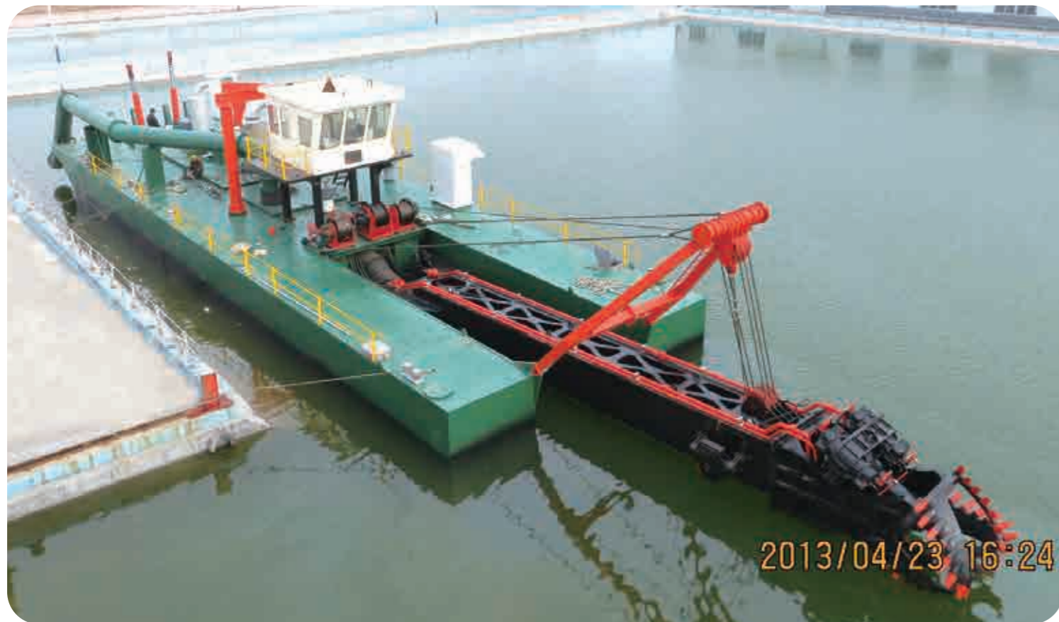
24inch HLC600 8000 m3/h hydraulic cutter suction dredger
